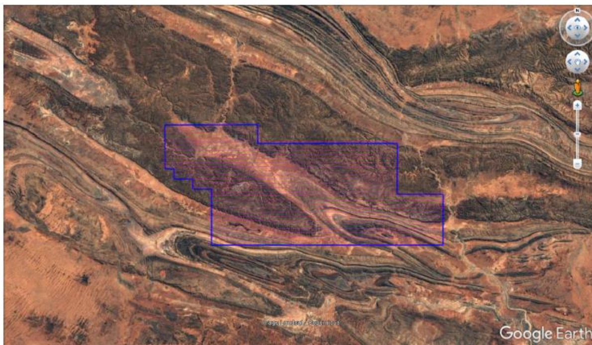
Figure 1 Airborne Gravity and Gradiometry Survey Area, 1181km of lines acquired at 750m line spacing (Xcalibur, 2021)
